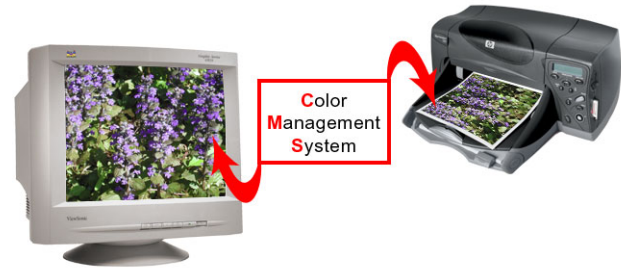
Figure 2 A CMS ensures that the appearance of the monitor matches the appearance of the print.
