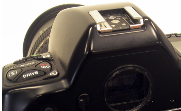
Hot shoe on an SLR camera where you can attach an additional flash unit.
